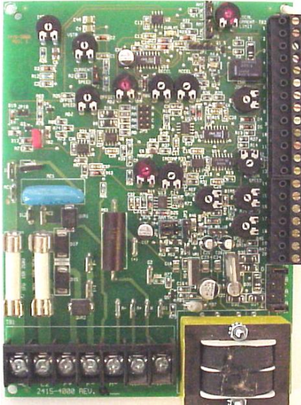
(1) Control Board for Non-Regen drives PN: 2415-4000
