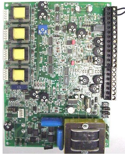
(8) Control board for Regen drives F3R5C and F3R5E PN: 6045-4005
