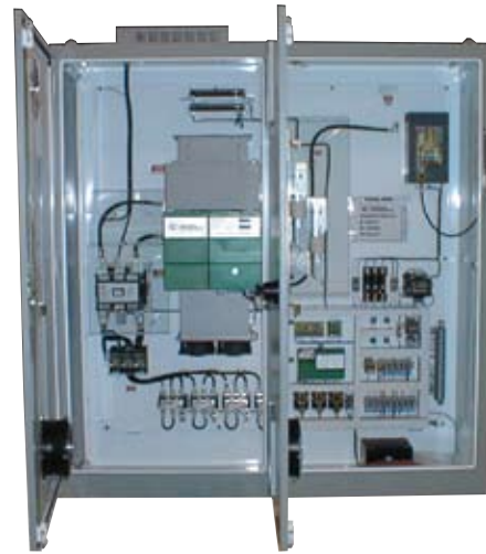
Nema -12 (PPBF), Ventilated Encl., 500 hp, 460 VAC, Non-Regen, Circuit Breaker, DC Contactor, Field Regulator
